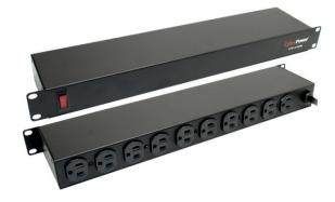
CyberPower's Power Distribution Unit (PDU) provides additional outlets for your rackmount power needs. The 1215RM offers 10 (ten) 15A rear-mounted outlets in the 19" 1U case. The rugged metal housing can withstand the most demanding environments and a 15' cord ensures compatibility for most rackmount applications. CyberPower PDU's can also be used for retail, security, POS, telecommunications, networking, audio/video displays, or anywhere dedicated power distribution is needed.
